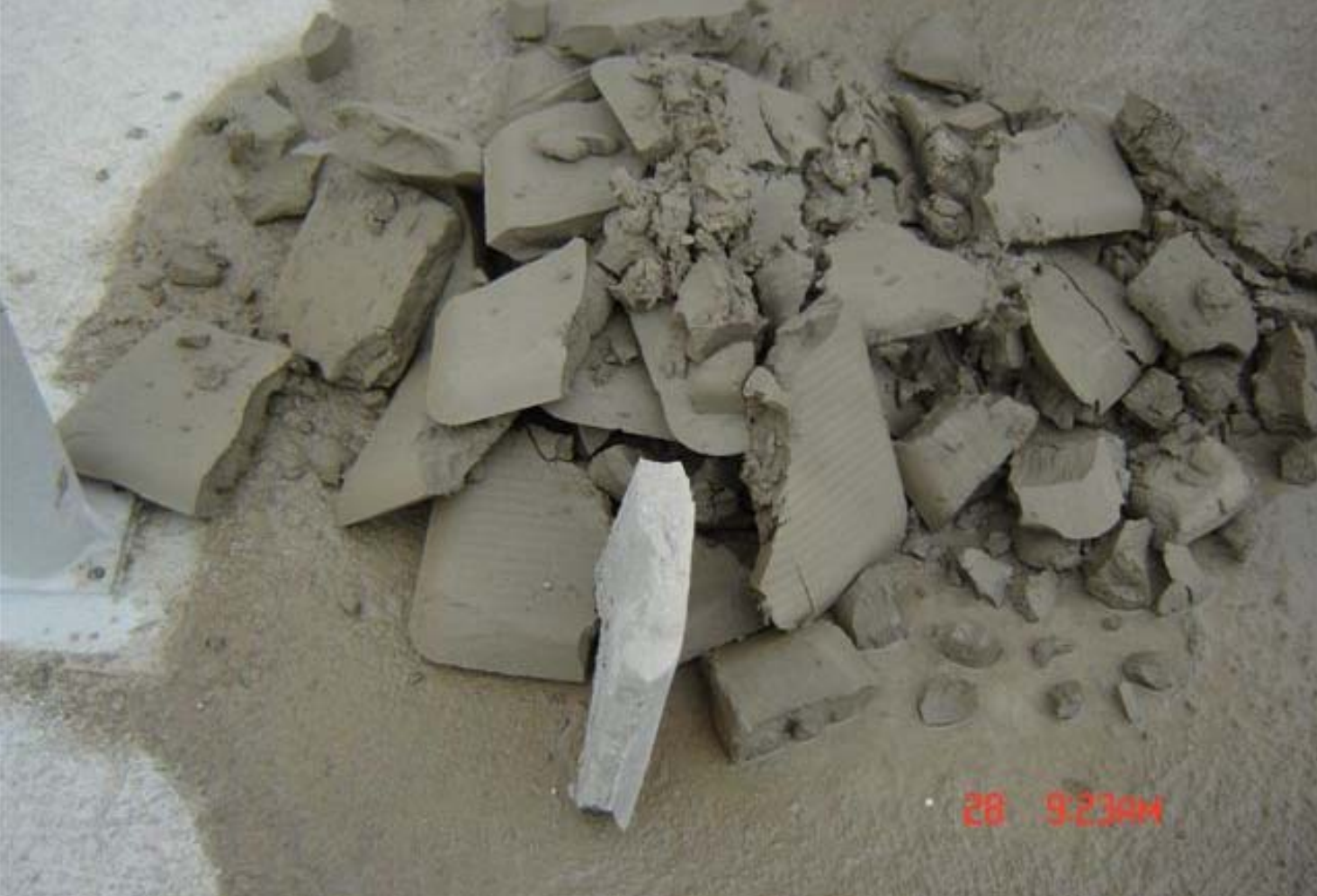
The dehydrated mud (Fig. 8) is dumped beneath the filterpress.
