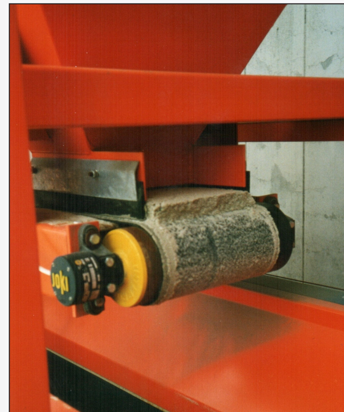
Here the dosing belt for the aggregate is shown, the dosing accuracy is very high due to the controlled volume on the belt.
