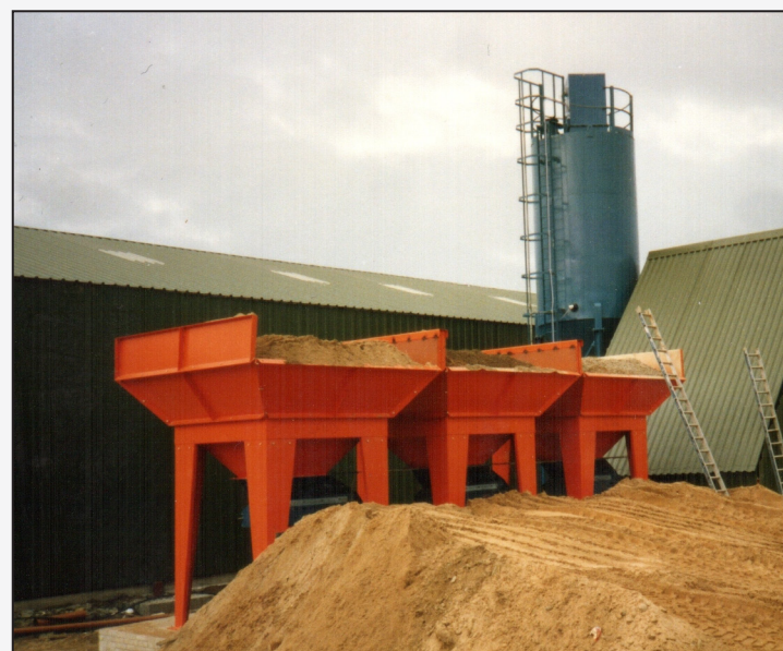
Stationary hoppers are used when the demand for one type of aggregate is used in the face-mix.
