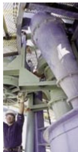
A further benefit is that the ReCyclone cone can be adjusted "on-the-run" for fine-tuning of the split to the secondary cyclone - there is no need to stop the plant to change spigots.
