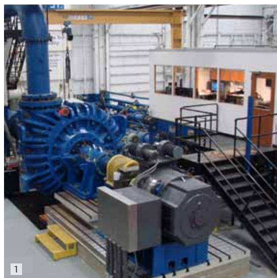
2: A Warman® 600 HTP pump being prepared for hydraulic testing. The massive rib reinforced casing and 102,000 lb (46,260 kg) bare weight illustrate the robust design and inherent safety of this 580 psi (4,000 kPa) rated pump
