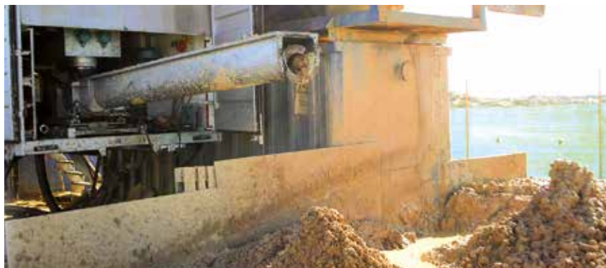
Installation of “high solid load” fines slurry sludge separation with conveyor technique
