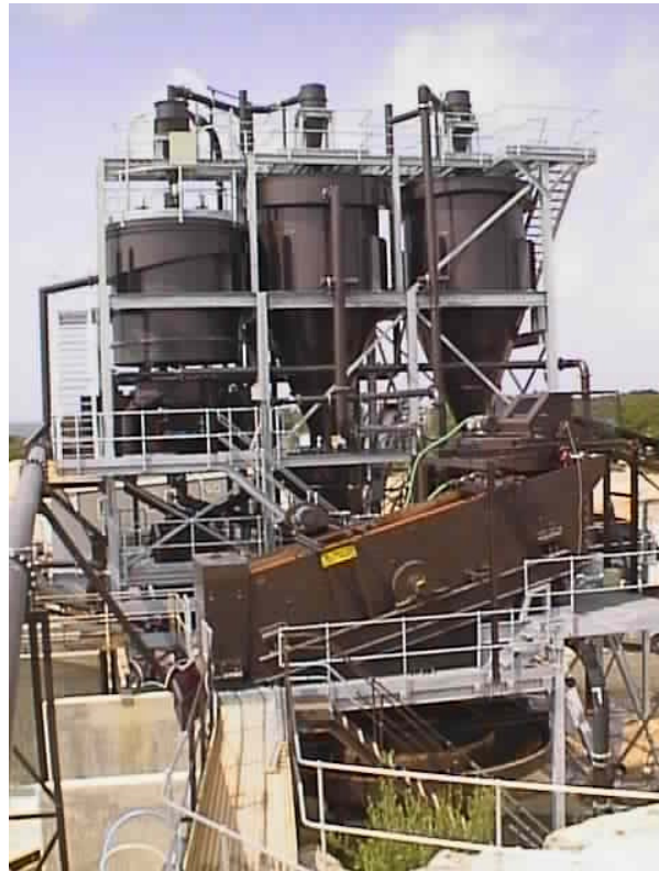
Dual In-Line Blending plant with two 3.0m T-Type Classifiers and DMS for lignite removal.
