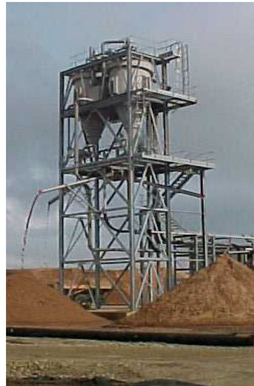
Twin 2.4m T-Type Classification System with lignite removal
