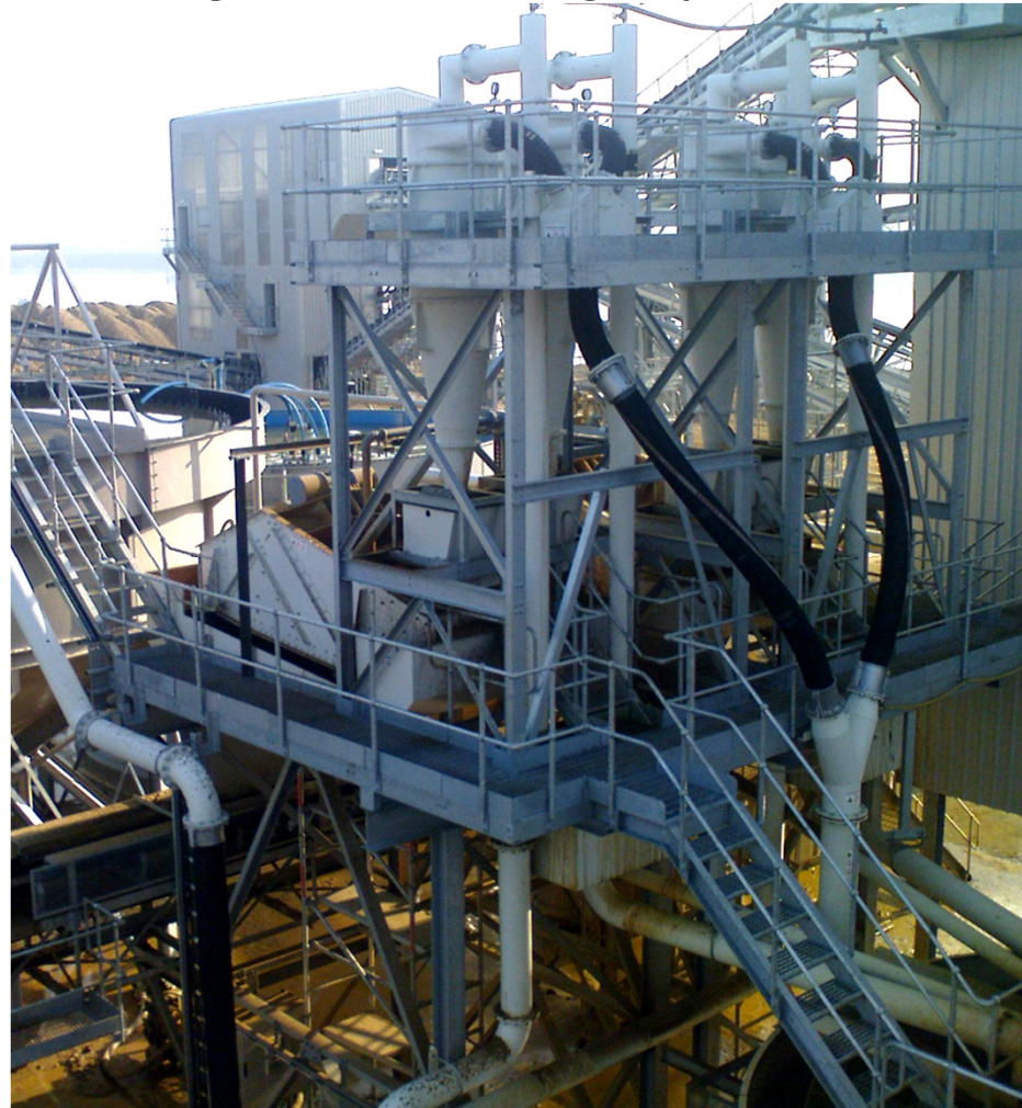
Primary sand washing & dewatering of 380tph of -5mm material Effluent Treatment by thickener & silt return onto dewatering screens.
